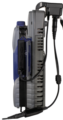
The headset adapter connects to the AVX-10K
