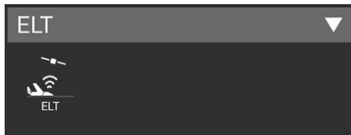
**121.5/243 BCN Modes** — Provides monitoring for 121.5/243 MHz swept tone short range Beacons and displays transmitter frequency, power and start/stop tone frequencies. Audio output is available.
