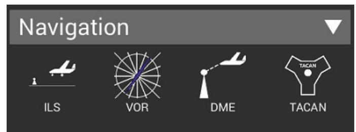
**ILS** — Provides simultaneous Localizer (with swept DDM), Glideslope and Marker Beacon Signals.
