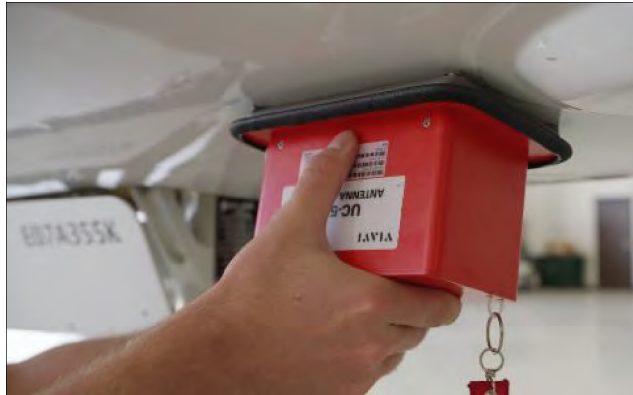
Figure 3-1 Coupler Test Setup
