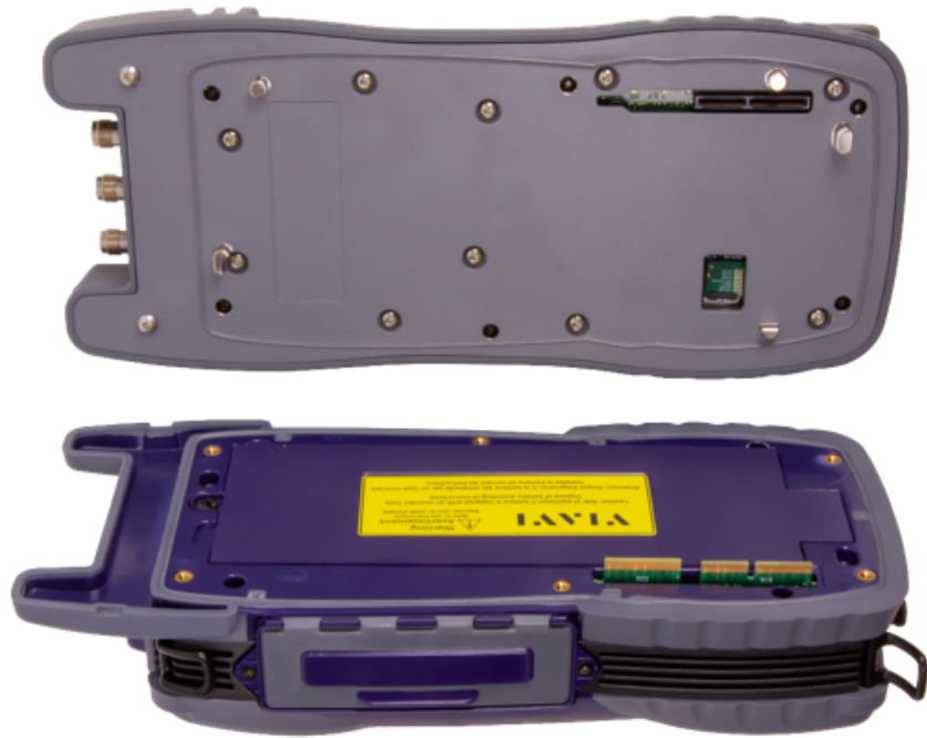
Figure 12-3 Battery Cover Removal
