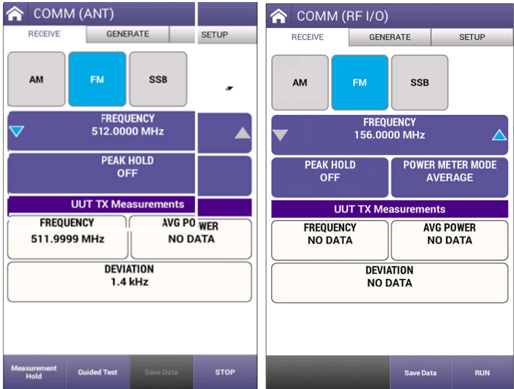
Figure 7-8 VHF COMM Frequency Modulation (FM) Receive
