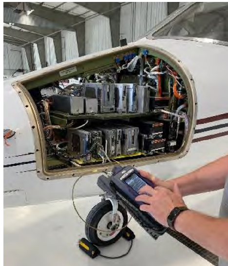
Figure 3-5 Direct to UUT Test Setup
