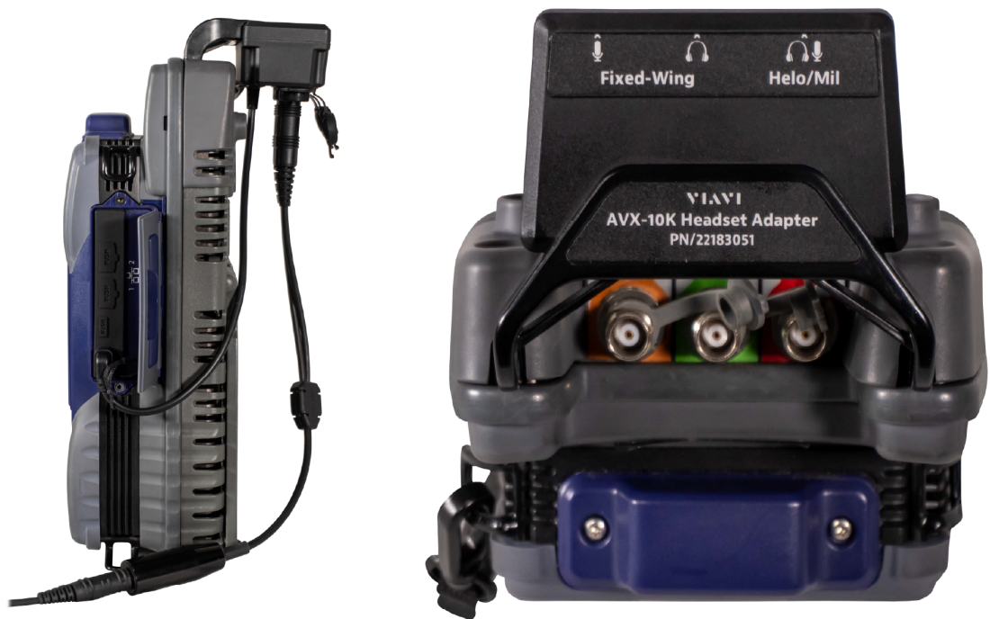
Figure 7-5 Enhanced COMMS Headset Adapter Setup
