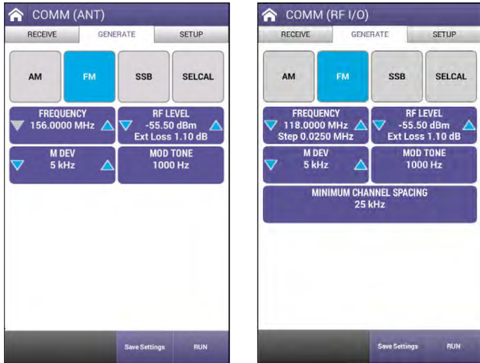
Figure 7-9 VHF COMM Frequency Modulation (FM) Generate
