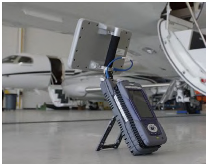
Figure 3-2 Over-the-Air Test Set-Up
