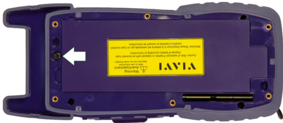
Figure 12-4 Battery Cover Screw Removal
