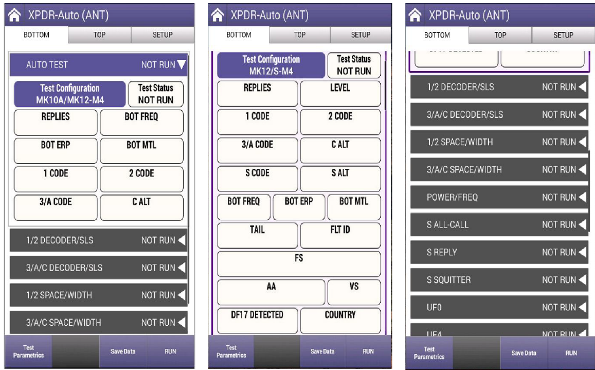
Figure 4-11 Mode 1/2 Transponder Test
