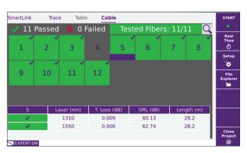
Integrated project management with Cable-SLM – up to 9996 fibers
