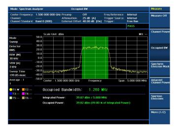
RF test — Occupied Bandwidth
