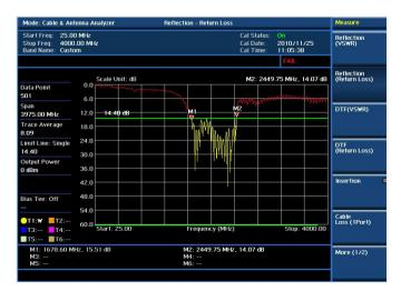
Cable and antenna test — Reflection
