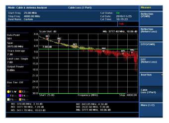
${\sf Cable} \, {\sf and} \, {\sf antenna} \, {\sf test} - {\sf Cable} \, {\sf Loss}$
