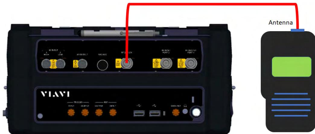
Figure 3-1 P25 Transceiver Test Setup Diagram
