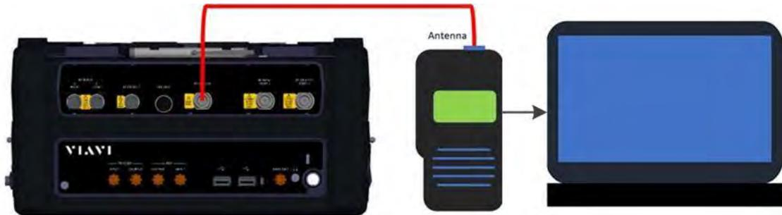
Figure 3-2 P25 Receiver Sensitivity Test Setup Diagram
