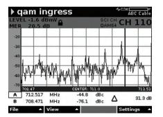
QAM Ingress test allows the technician to see what is going on underneath a live digital carrier which is usually not viewable due to the presence of the "havstack".
