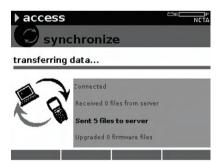
By synchronizing the DSAM, a technician can receive updated meter information as well as send back saved test data for historical record keeping and Home Certification tests.
