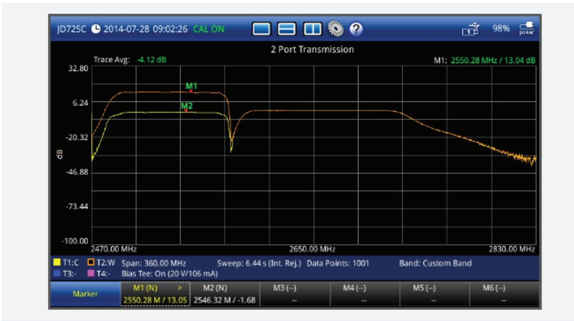
Figure 4: Insertion Loss Test view
