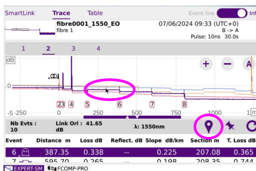
Figure 72 OTDR Trace - New event
