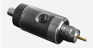
Simply screw the probe into a KS port on the distribution tap, connect the field meter to the test port, then press the button on the side of the probe. If the headend ingress displayed decreases by 4 to 6 dB when the button is pressed, the source of the ingress is farther from the node than the test point. Ingress that does not decrease is entering the system nearer to the node than the test point. The I-Stop probe has little or no visible effect on forward path signals.
