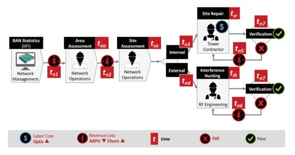
Conventional maintenance process for interference
