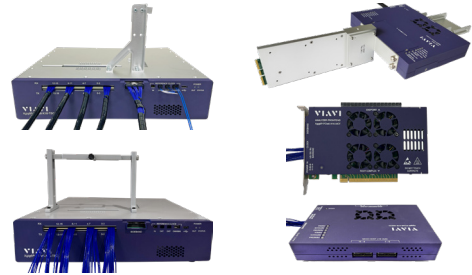
Test Stands and Interposers in multiple form factors
