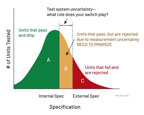
Figure 1. Measurement impact
