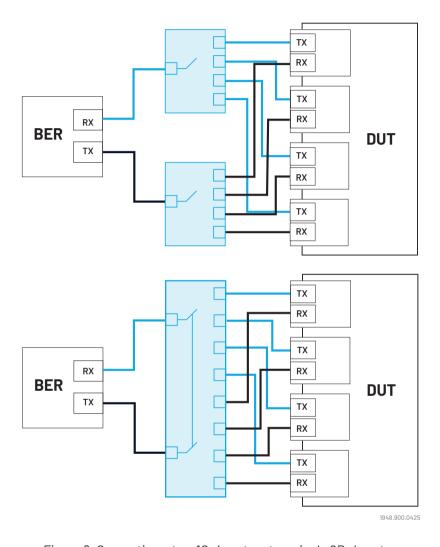
Figure 8. Converting a two 1Cx4 system to a single 2Dx4 system
