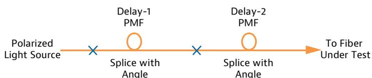
Figure 2: Broadband source with Lyot depolarizer implementation
