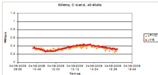
Figure 5: Inter-comparison results between the new VIAVI High-Res PMD and a JME-based solution
