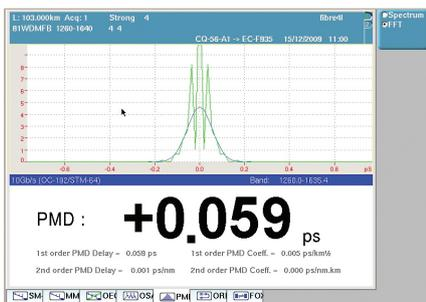
Figure 4: PMD measurement of a 103 km buried fiber link
