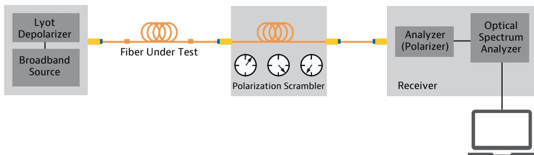
Figure 3: Typical schematic of the elements in the high resolution Fixed-Analyzer solution
