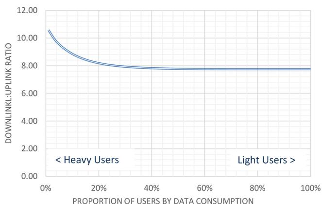
Figure 2. Downlink/uplink ratio by proportion of users
