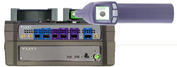
Figure 3: OTDR Port Inspection
