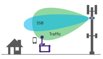
5G EMF code selective measurement on traffic beams over a high-speed data transmission
