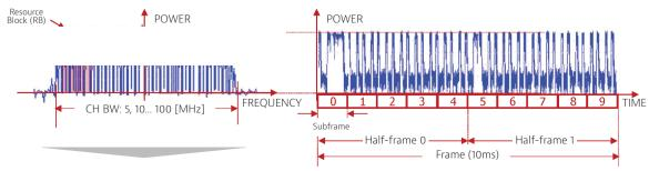
3GPP 5G NR Signal Channel and Frame Structure
