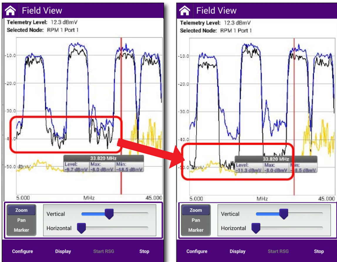
Left: Noise visible between the active upstream carriers
