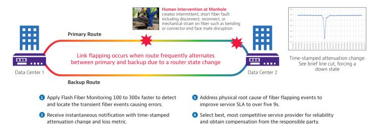
This innovative, VIAVI patented feature is uniquely designed to assist in troubleshooting network flapping. It provides a time stamp of the attenuation event to be correlated to route flapping or error events in your NMS or router topology table. **Customers are able to see the location of these events and advance the troubleshooting process dramatically by detecting and locating ISDFs caused by flash attenuation events, which is especially critical for high-speed rates.**
