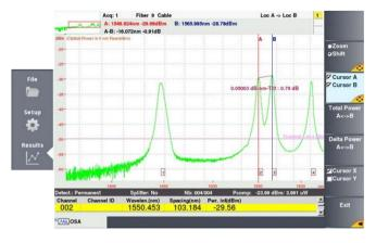
Fig. 13 Example of Delta Power measurement
