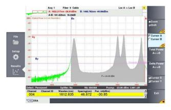
Fig. 12 Example of Total Power measurement
