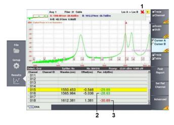
Fig. 17 Displaying multiple traces
