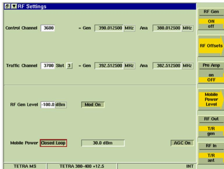
Fig. 5-22 TETRA MS RF Settings Tile - Channel Plan Selected
