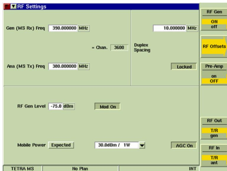
Fig. 5-23 TETRA MS RF Settings Tile - No Channel Plan Selected
