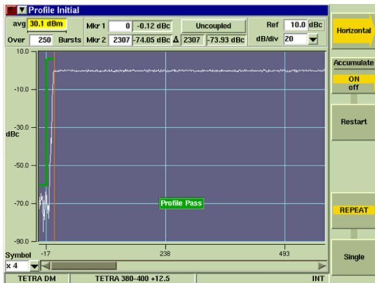
Fig. 9-25 TETRA DM Power Profile Initial Tile - Maximized View
