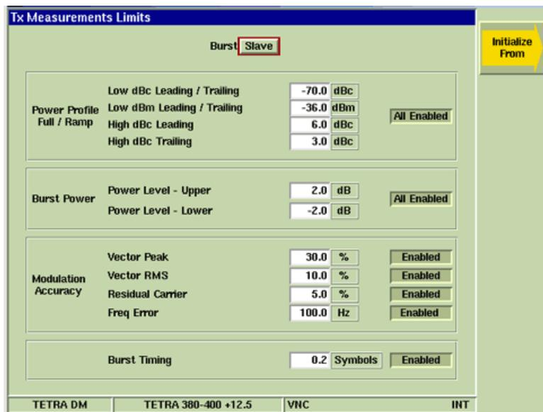
Fig. 9-13 TETRA DM Tx Measurements Limits Configuration Tile
