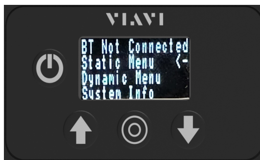
Figure 1-3 OSPREY Front Panel Display / Control
