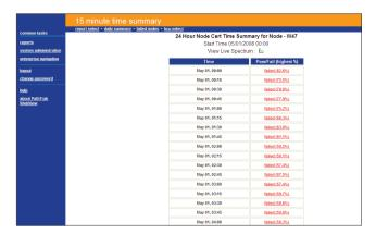
The time-over-threshold report displays the percentage of time a frequency exceeds the selected Threshold T1-4 for a particular time window. It is used to measure carrier performance based on the percentage of time it remains in alarm state.
