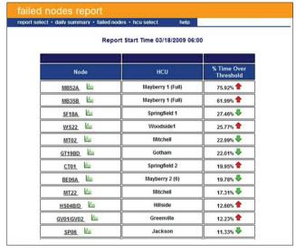
WebView server software automatically ranks node RF upstream performance  $\,$ based on quantitative test data gathered by PathTrak
