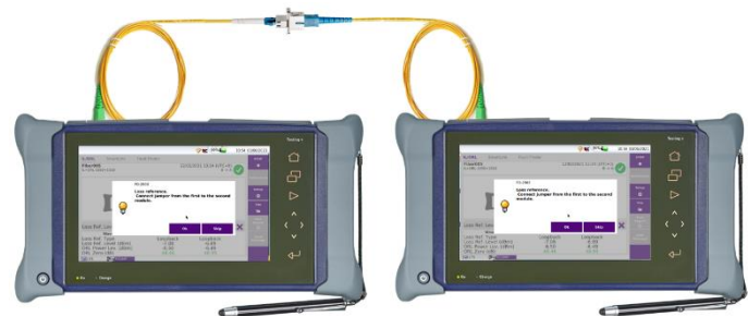
Figure 9: "Two-cable" Side by Side Reference
