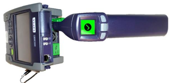
Figure 3: OTDR Port Inspection
