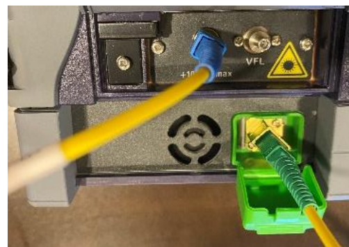
Figure 7: OTDR module connection to mainframe power meter
