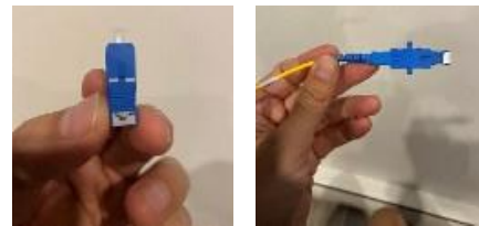
Figure 8: OTDR module connection to non-reflective termination
