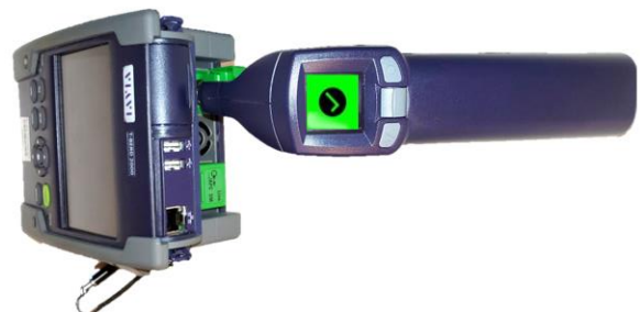
Figure 3: OTDR Port Inspection
