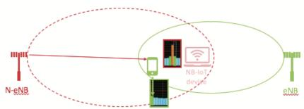
A similar situation of potential signal pollution could take place on the uplink path if the NB-IoT device originates an excessive level of PSD boosting or even an excess of signal repetition to better reach the base station for data transmission. This could result in desensitizing the adjacent LTE base station and could cause a significant decrease in the quality of service being delivered (similar to a near-far phenomenon).
