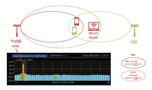
Technicians should analyze any potential changes to the coverage area of the LTE base station when the NB-IoT signal service is activated from an adjacent base station and its associated PRB is actively transmitting.
