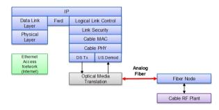
Figure 1 Current - Centralized Access Architecture
