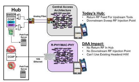
Figure 6 RF Test Points Removed from Hub with DAA
