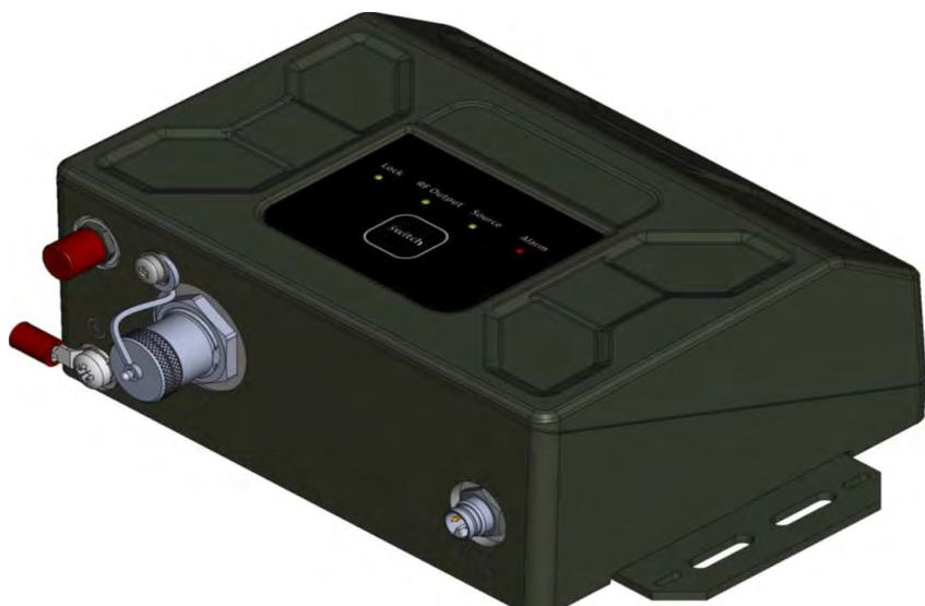
The RSR Transcoder 2.0 enclosure operates from a 7V to 36V DC power supply. The unit can accept PVT fixes over its RS-232 or USB serial ports via its built-in NMEA parsing capability, in addition to accepting PVT fixes via standard SCPI commands. Simulation motion control commands can be stored in internal EEPROM and used to
