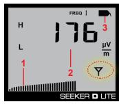
Tagged Signal Detected (High Frequency)
