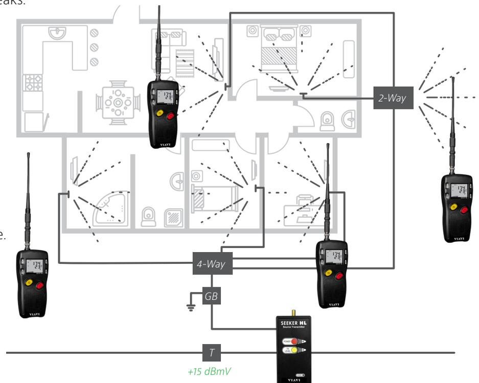
Using the Seeker HL with its source transmitter allows the technician to detect leakage levels at an otherwise unheard of sensitivity down to 0.1  $\mu\text{V}/\text{m}$ . The user may set the output level to 60 dBmV for home certification, but also has the option to reduce the level to 40 dBmV should the subscriber network prove to be too porous for pinpointing the location of a leak at the higher transmit level.
