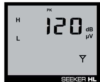
Within the input level setting mode, the PK icon in the upper middle side of the screen flashes.
