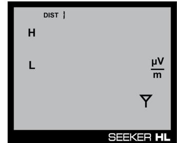
The image displayed to the right represents the normal measurement mode of the leakage detector set to 3 meters, as indicated by “DIST 3”.
