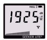
In this mode the **Antenna** icon on the display blinks to show the Signal Level display is selected.
