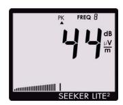
In the Peak Hold display, the **PK** icon at the top of the display will blink if the Peak Hold function is off. The **PK** icon will be constantly displayed if the Peak Hold function is on.
