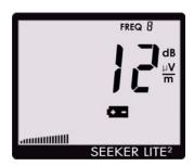
In this mode the **Battery** icon on the display will blink to show the Battery Charge Level display is selected.
