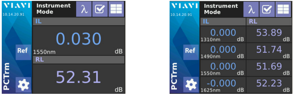
Simple large display shown in single and multi-wavelength mode. The capacitive touchscreen enables quick and efficient navigation.
