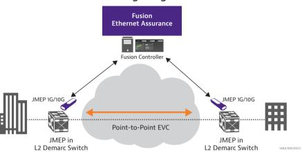
Site-to-Site Testing Using smart SFPs
