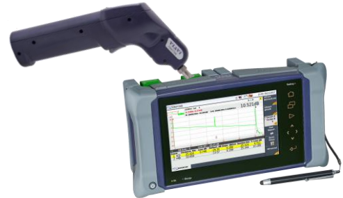
Figure 3: OTDR Port Inspection
