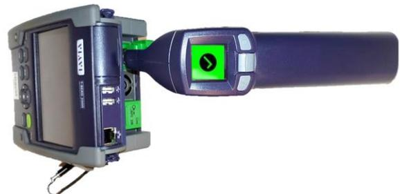
Figure 3: OTDR Port Inspection
