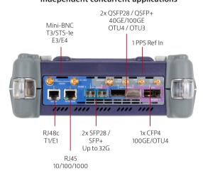
2x SFP+/SFP28 1-10-25G Ethernet LAN/WAN OTN 1-1e/2/2e STM-1-64 & OC3-192 Fibre Channel: 1,2,4,8,10,16G, 32G FC CPRI 614M – 10.1, 24.3G
