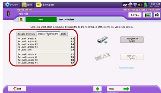
Figure 9: Optical Power (dBm) Results (100GBASE-LR4 optics)
