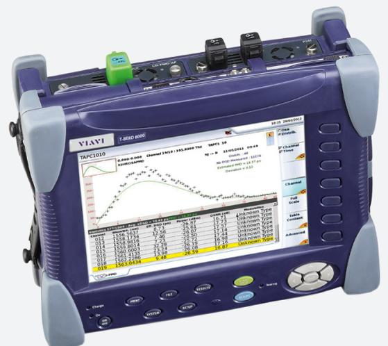
Smart and easy, the I-PMD test solution automatically identifies live channels and uses a measurement grid to perform PMD, channel power/frequency, and I-OSNR tests in a single scan.
