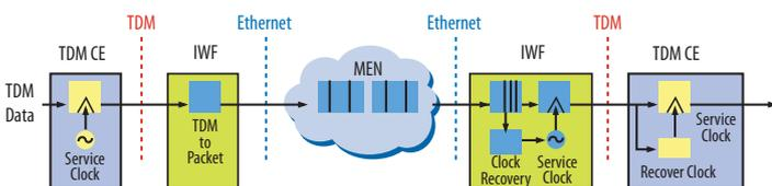
Figure 2. Network Reference Model for Timing Distribution over Packet Networks
