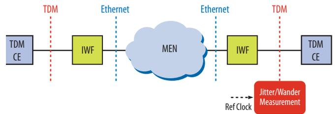
Figure 6. TDM Jitter/Wander Test Measurement Setup
