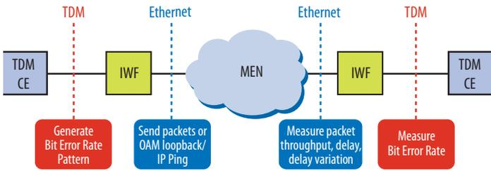
Figure 5. Basic TDM/Packet Test Setup
