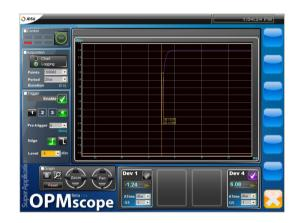
After the trigger event takes place, the data appears as shown in Figure 6. The markers here indicate that it took approximately 0.68 ms for the signal to rise from -4 to 3 dBm.
