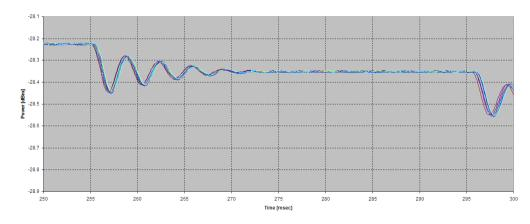
Figure 1: Measuring settling time in the optical domain
