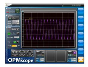
Figure 5: Real-Time Sinusoidal Signal measurement
