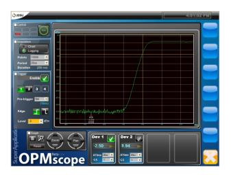
Figure 3a: Optical Step Function measurement in MOPM-B1 Gain Stage 1
