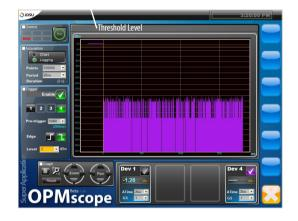
Figure 8 shows the measurement results. Note the pretrigger data points as well as the trigger level. Post processed data indicates that it took approximately 0.098 ms for the signal level to drop from 3 to -45 dBm.
