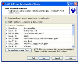
6. To set TDM as the 860 DSP's or 860 DSPi's home page, right-click the 860 DSP or 860 DSPi in the Navigator window. From the floating menu, select **Configure**, then select **Web Browser Parameters**.
