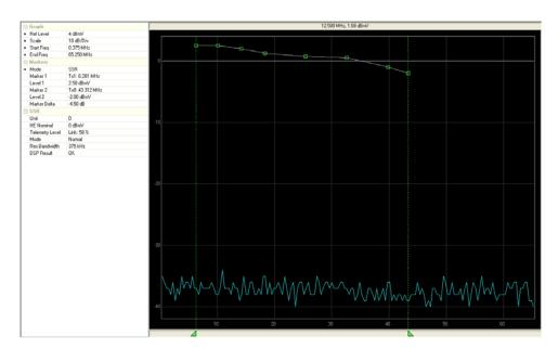
There are two different modes of reverse sweep report: sweep and compare. The report mode is selected on the 860 DSP at the time the test is performed. The sweep graph has a light blue ingress trace and a sweep graph with up to eight green squares or red X's connected by a white line. The compare graph has two ingress line graphs (light and dark blue).
