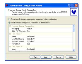
The Forward Sweep Parameters configuration is a carry-over feature from the 860 DSP and 860 DSPi field analyzer, and as such, is not applicable to the 860 DSPr headend analyzer configuration.
