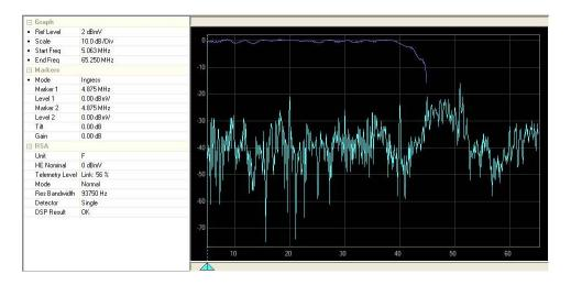
test is performed. The sweep graph has a light blue ingress trace and the sweep trace has a dark blue line.
