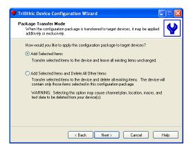
configuration package to the 860 DSP or 860 DSPi and delete any other files on the 860 DSP or 860 DSPi. At the end of the transfer process, the only files and information on the 860 DSP or 860 DSPi will be the files and information contained in the configuration package. This option is useful for ensuring that 860 DSP's or 860 DSPi's are configured to a standard and that no unauthorized or unacceptable files are included on them.
