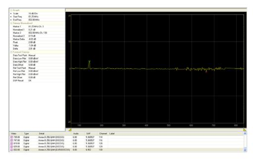
reference and the current levels (may be the same test point at a different time, or a different test point down the line in the network).
