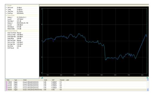
The Scan Data View Graph compares the levels at two different points in the cable system. In this view, the light blue line is a plot of the measured scan of all channels. The dark blue line is a reference scan that was previously taken at a different place on the cable network and stored for reference purposes.
