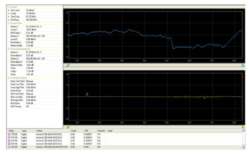
The Split View Graph shows both the Scan Data View (Top) and the Normalized Data View (Bottom) on the same graph.
