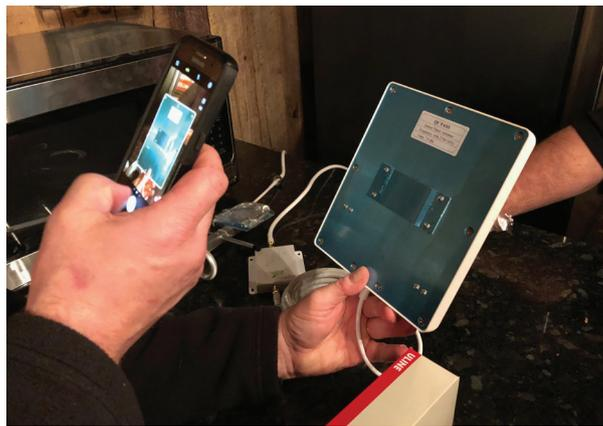
Repeater that caused the interference
