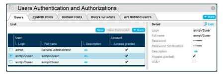
SNMP v2: the ONMSi user login must be the same as an SNMP v2 community SNMP v3: the ONMSi user login must be the same as the SNMP user name
