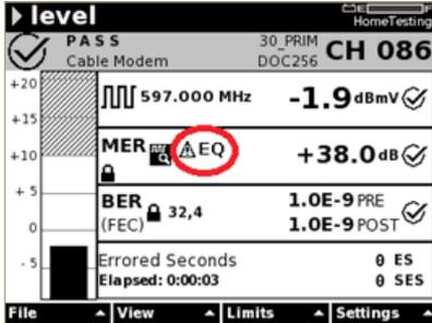
Equalizer warning appears in the signal measurement screen indicating an equalizer-related issue
