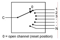
Figure 2: Single-Common Configuration
