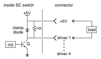
Figure 12: Sample Driver Application: Electrical Equivalent of Driver
