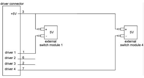
Figure 10: Switch Setup without TTL
