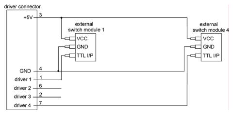
Figure 11: Switch Setup with TTL
