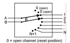
Figure 4: Single-Step Dual-Common Configuration
