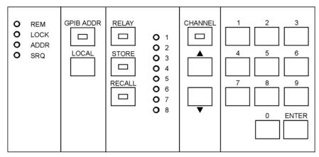
Figure 8: Operating Keys and Status LEDs
