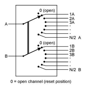
Figure 3: Dual-Common Configuration
