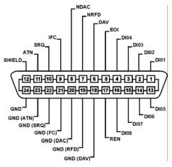
Figure 15: GPIB Pin Assignment
