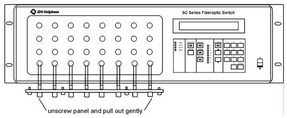
Figure 14: Removing the Connector Panel
