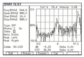
Figure 4.0 The 3500 distance to fault and VSWR test screens
