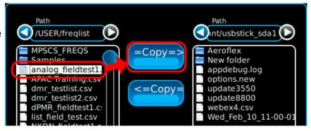
To copy the modified frequency list back onto the 8800SX or to other units, reverse this process.
