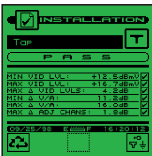
The results are displayed in a list indicating which parameters are out of tolerance. If all levels are within limits, a “3” will be in the right far column. If any parameter is out of tolerance an “x” will be shown.
