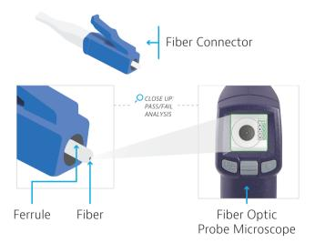
Debris on an end face is typically 2 - 20µm and can only be seen with a fiber optic probe microscope.
